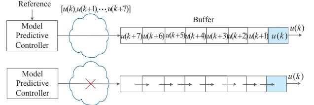
Figure 5: Buffered Actuation Mechanism
