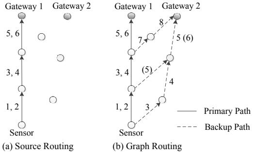
**Figure 2: Source and Graph Routing**
