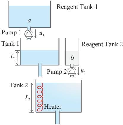
**Figure 3: Exothermic Chemical Reaction Plant**
