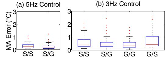
**Figure 13: Maximum Absolute Error for Temperature Control with Noise Strength = -73 dBm.**
