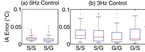
Figure 10: Integral Absolute Error for Temperature Control with Noise Strength -74 dBm.
