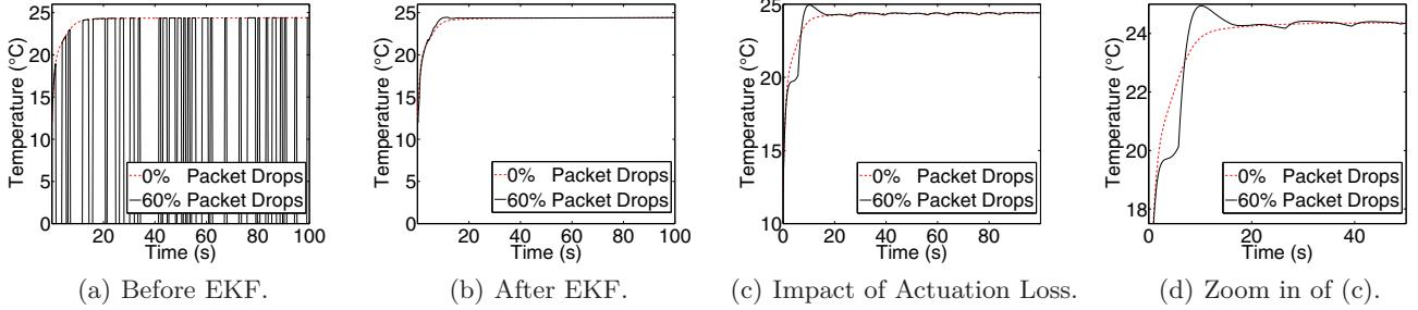
**Figure 6: Results of EKF and Buffered Actuation:** (a) Temperature measurement before EKF and with 60% sensing packet drops; (b) Temperature after EKF and with 60% sensing packet drops; (c) Temperature measurement with 60% actuation packet drops; (d) Zoom in of (c).
