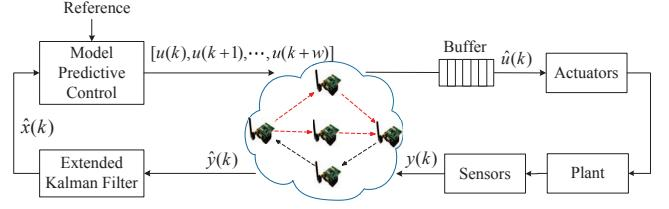
**Figure 1: System Architecture:** Sensor measurements from sensors are transmitted wirelessly to the observer, which generates estimated system states. The controller takes estimated system states and computes actuation commands, which again are transmitted to actuators wirelessly. We introduce a buffer for actuators such that we can reuse previously buffered actuation inputs when packet drops happen.
